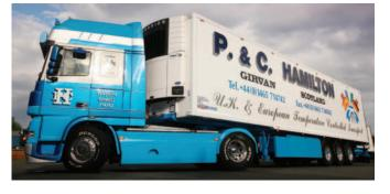
"Being able to operate across EU borders is a necessity for this trailer, so we specified it to meet Class C ATP standard to operate with a setpoint between +12 and 20°C," says Hamilton.
